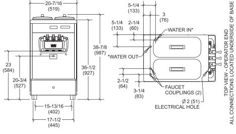
NOTE: 1. FIGURES IN PARENTHESES INDICATE MILLIMETERS. \* WATER COOLED UNITS ONLY
